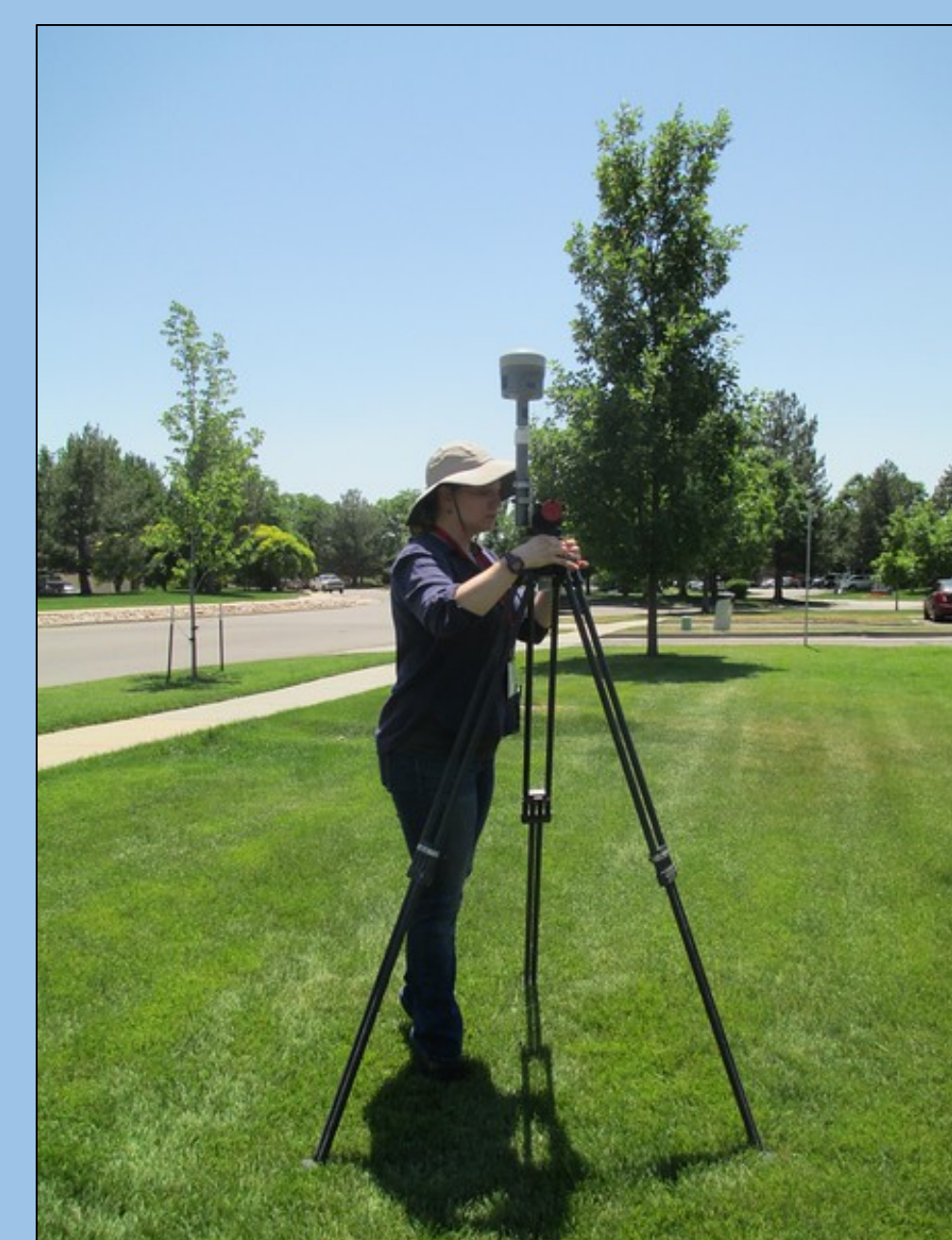
Above: Geo-Launchpad Polar Team went into the field to measure snowpack of the St. Mary's Glacier using two types of GPS: PPK and RTK. Left: Laura Fakarhai performs leveling procedures on a GPS station.
